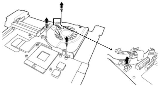
Figure 4-43 Removing screws securing FAN and disconnecting cable
